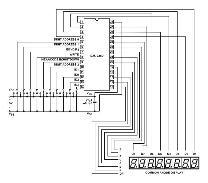
FIGURE 19. FUNCTIONAL TEST CIRCUIT #2
