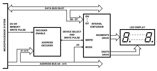
FIGURE 9. ICM7228A/B MICROPROCESSOR SYSTEM INTERFACING
