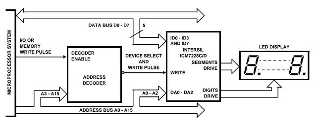
FIGURE 10. ICM7228C/D MICROPROCESSOR SYSTEM INTERFACING
