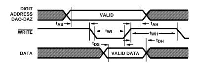
FIGURE 3. ICM7228C/D WRITE CYCLE
