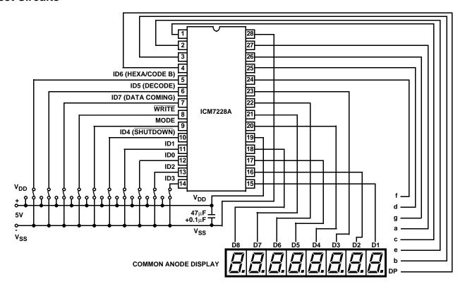
FIGURE 18. FUNCTIONAL TEST CIRCUIT #1
