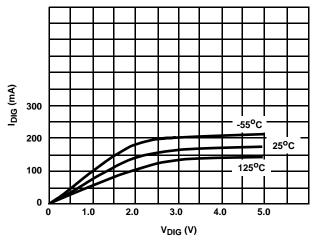
FIGURE 7. COMMON CATHODE DIGIT DRIVER  $I_{\mbox{DIG}}$  vs  $V_{\mbox{DIG}}$
