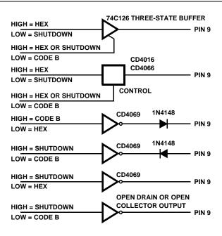
FIGURE 17. ICM7228C/D PIN 9 DRIVE CIRCUITS
