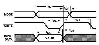
FIGURE 1. ICM7228A/B WRITE CYCLE
