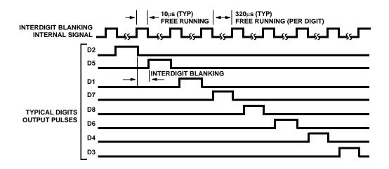
FIGURE 4. DISPLAY DIGITS MULTIPLEX (COMMON ANODE DISPLAY)
